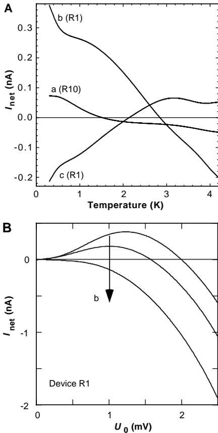
**Fig. 2.** (A) Temperature-induced current reversal. Net current versus temperature for devices R10 (curve a) and R1 (curves b and c) at fixed gate voltages as indicated by the corresponding letters in Fig. 1.  $U_0 = 1$  mV in all cases. The temperature was measured with a calibrated Ge sensor that was heat sunk in the same way as the device. (B) Net current versus rocking amplitude for device R1 at the gate voltage denoted by point b in Fig. 1B at (from top) 0.6, 2, and 4 K.
