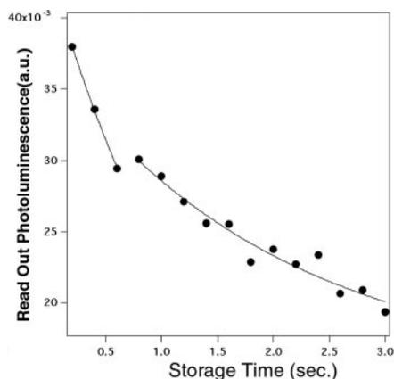
**Fig. 5.** Low-temperature (3 K) integrated intensity of the readout signal as function of time for a forward bias of 0.5 V. The lines are exponential fits to the data. The storage time extrapolated to the average noise level (on this scale,  $6 \times 10^{-3}$ ) is  $\sim 10$  s.
